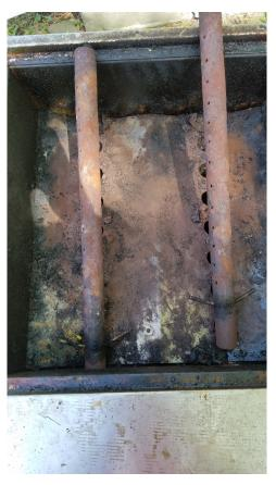
4. Remove the burner once clear of hole in the front wall.
