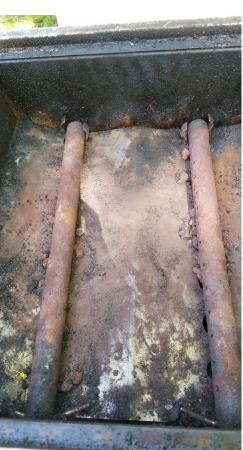
3. Pick up the burner just in front of the opened bracket and gently lift at an angle - carefully sliding the front portion out of the hole in the front wall
