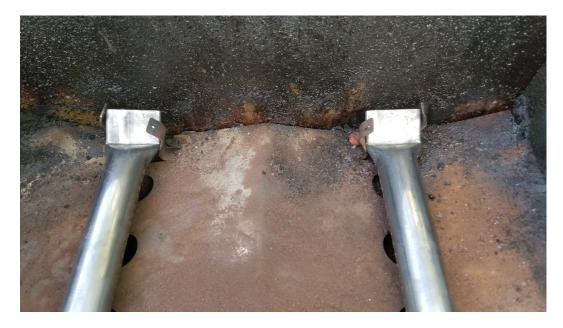
9. Replace lava rock in single layer over burners (about 6-7 lbs. per section) completely covering the bottom of the section.
